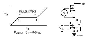
Figure 9. Gate Charge Characteristic
