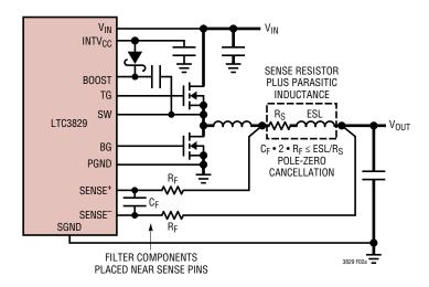
(2a) Using a Resistor to Sense Current
