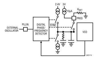
Figure 16. Phase-Locked Loop Block Diagram
