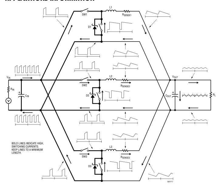
Figure 17. Branch Current Waveform
