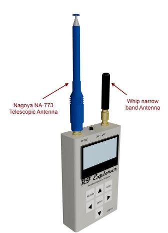
RF Explorer includes one antenna for standard models, or two antennas for ISM Combo, 3G Combo and Wifi Combo models.
