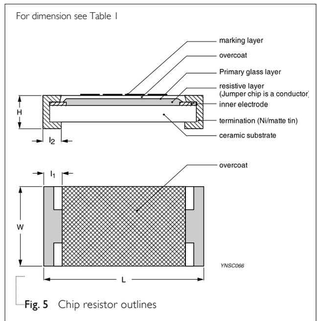
Fig. 5 Chip resistor outlines
