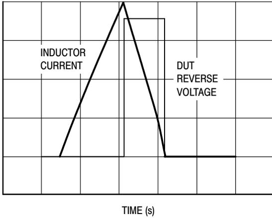
**Figure 11. Typical Voltage and Current UIS Waveforms**
