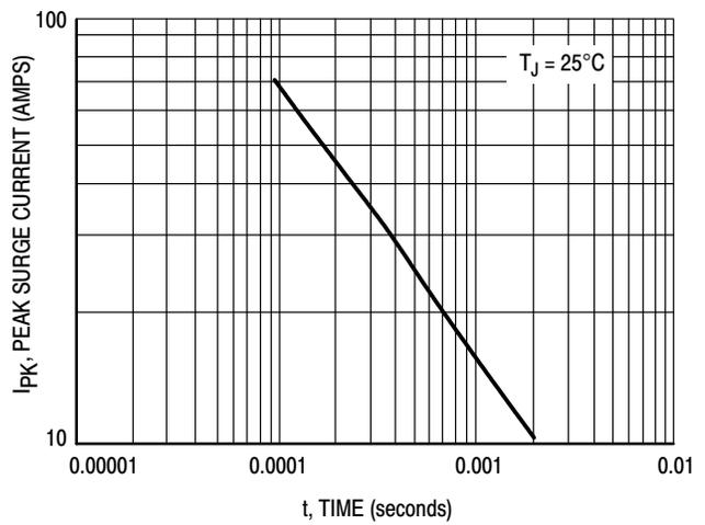
Figure 8. Typical Unclamped Inductive Surge
