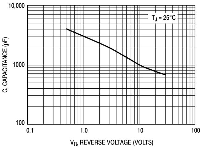
Figure 7. Typical Capacitance
