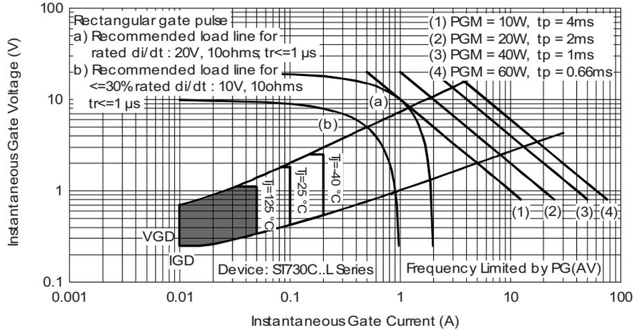
Fig. 11 - Gate Characteristics
